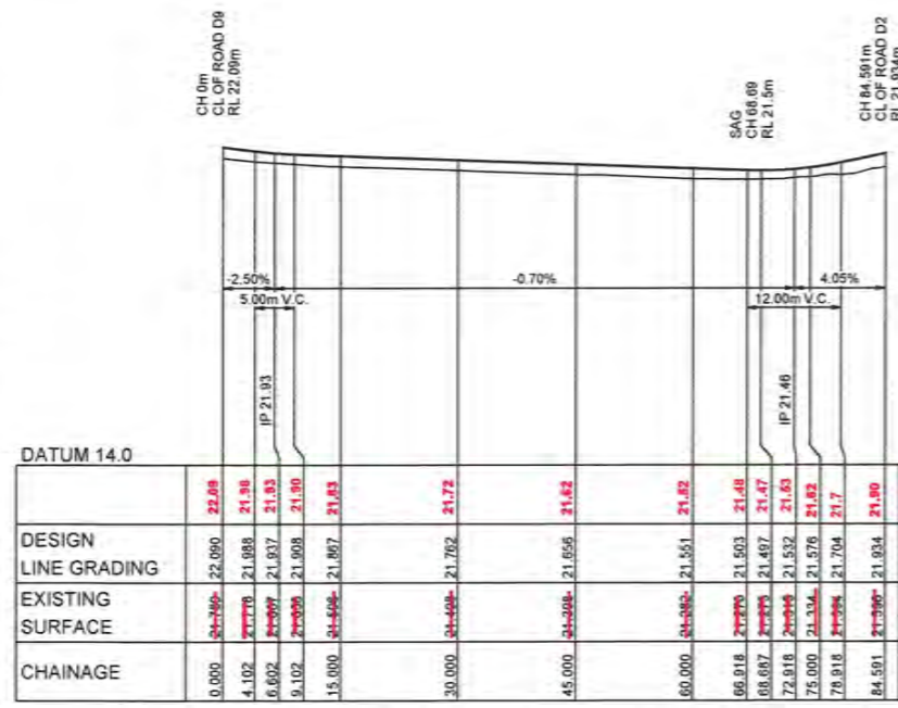
LONGITUDINAL SECTION - KAMALA STREET (ROAD D5) HORIZONTAL SCALE 1:500 VERTICAL SCALE 1:100
