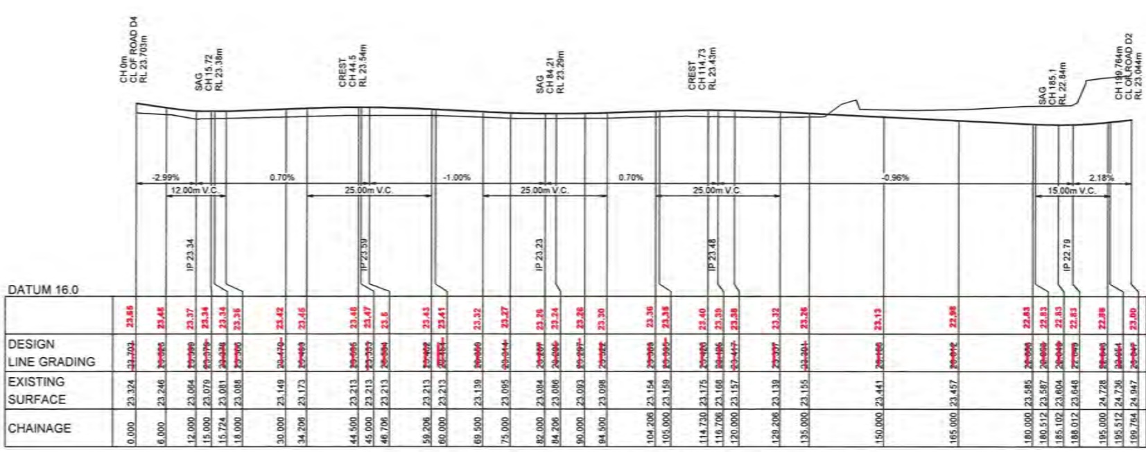
LONGITUDINAL SECTION - WOODRUFF STREET (ROAD D7) HORIZONTAL SCALE 1:500 VERTICAL SCALE 1:100
