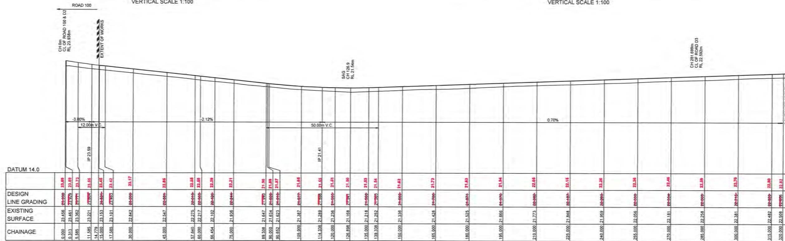
LONGITUDINAL SECTION - JACKWOOD CRESCENT (ROAD D1) HORIZONTAL SCALE 1:500 VERTICAL SCALE 1:100
